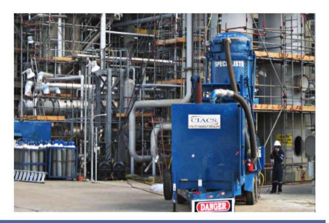
CIACS presently owns a fleet of vacuum units, which provides clients with the level of reliability and flexibility they deserve. These units are all capable of Nitrogen Recirculation with a dust control mechanism. Unlike some older vacuum units, all CIACS' vacuum units are modified for the filling of containers while vacuuming. We have the right vacuum to suit any job.
