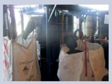
CIACS offers three levels of vibration screening capabilities. The system separates up to three sizes of material and also removes the dust and fines. All dust is contained and can be setup to vacuum airborne dust.
